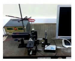
**Setup for Raman Spectrometer**
